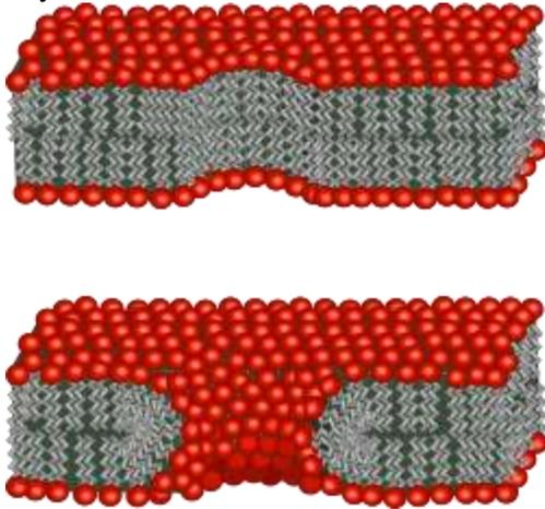
Schematic cross-section showing the theoretical arrangement of lipids in a hydrophobic pore (top) and a hydrophilic pore (bottom).
