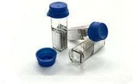
Cuvettes for in-vitro electroporation. These are plastic with aluminium electrodes and a blue lid. They hold a maximum of 400  $\mu\text{l}$ .
